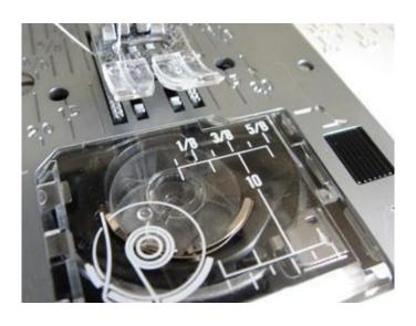
Faster to thread up, can see bobbin level, no oiling required
